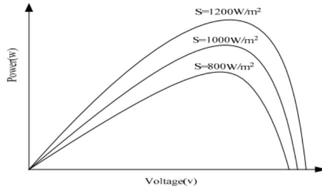
Fig.3.7: PV power characteristic for different irradiation level [55]
