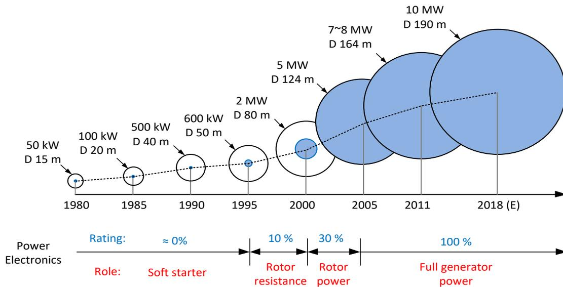
**Fig 0.3 Evolution of wind turbine size and the power electronics seen from 1980 to 2018 (estimated). Blue circle: the power coverage by power electronics [34].**
