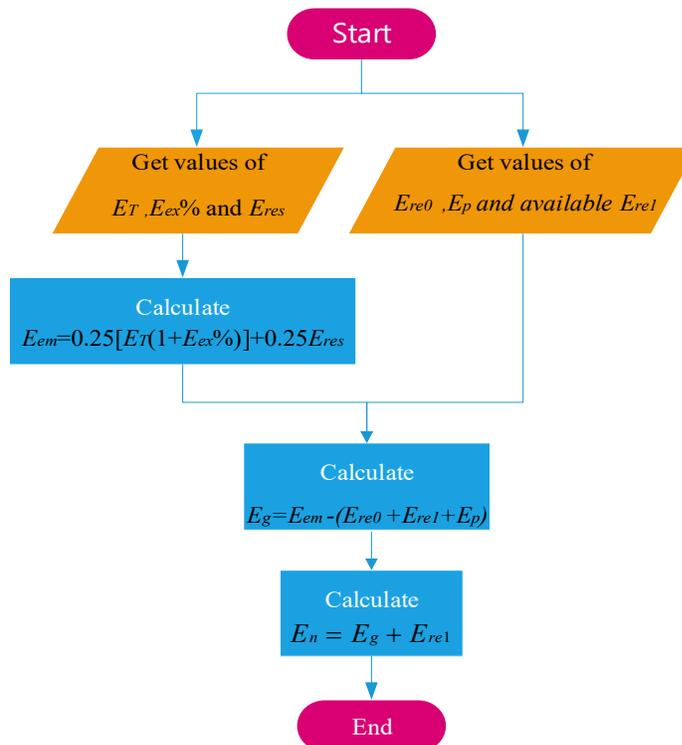
**Fig.4.1: Proposed algorithm for the emergency system**
