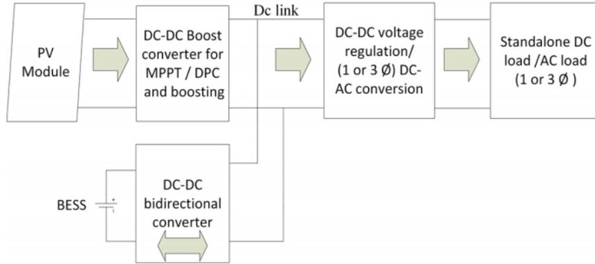
Fig.3.9: General Block Diagram of PV Standalone System [59]
