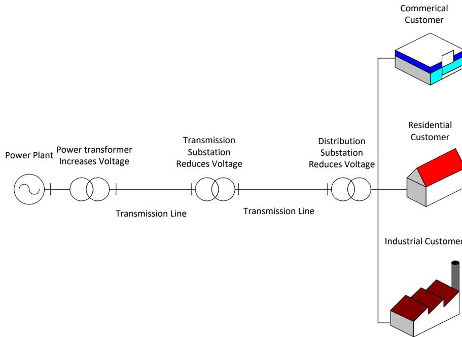
**Fig 0.1 A typical electric-power distribution grid [28]**
