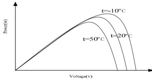
Fig.3.8: PV power characteristic for different ambient temperature level [55]
