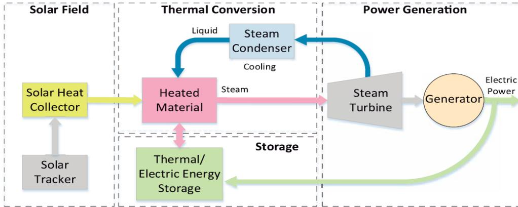
Fig. 3.6: Block diagram of a concentrated solar power system [54].
