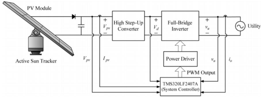
Fig.3.10: Configuration of grid-connected PV generation system [60]
