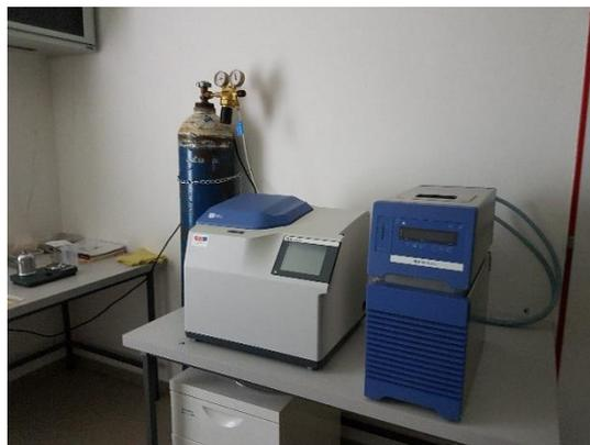
Figure 12: Calorimeter IKA C6000
