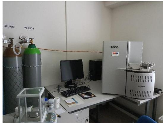
Figure 13: Elementary Analyser LECO CHN628
