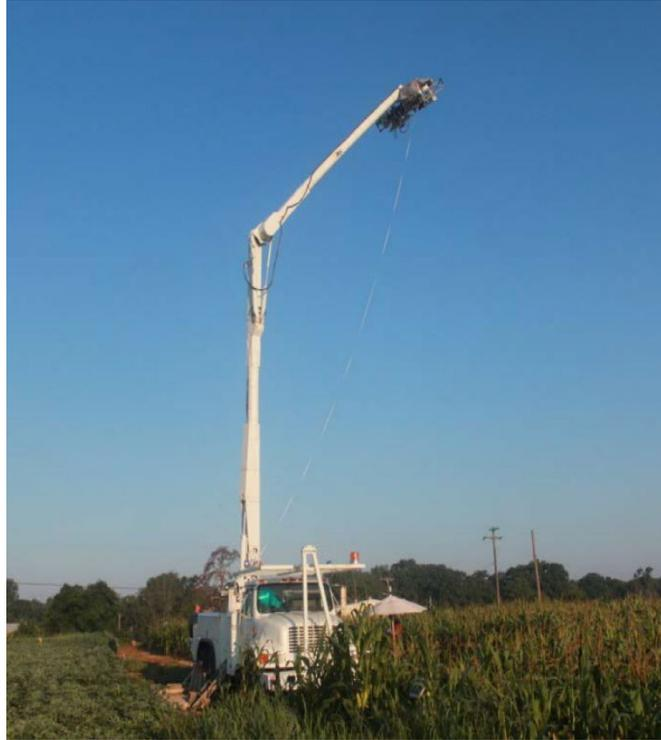
**Figure 10.** The ComRAD Microwave Instrument System – measuring the RVI.
